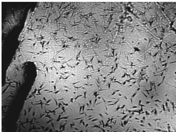
Fig. 1. Preferential dissolution by an acidic solution of neutron-induced fission tracks in a natural fluoroapatite.
